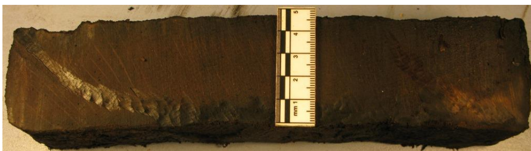
Figure 33 Photograph of dendro sample 3 from timber 22 showing the knotty nature of the timber on right
