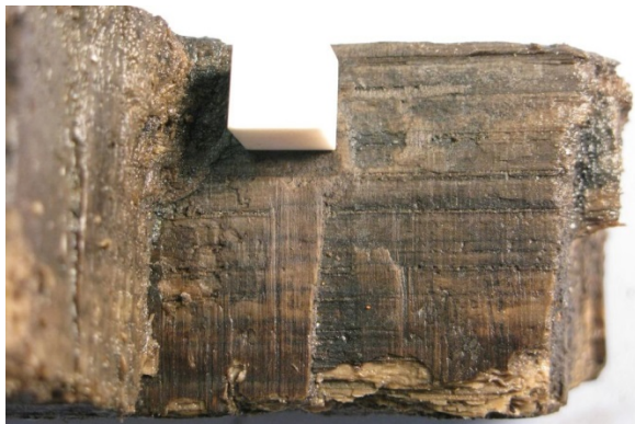
Figure 14 Photograph of saw marks on timber 3. Scale=1cm
