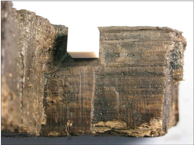
DP34 - Timber 3, Saw Marks - Hi Res Photo
