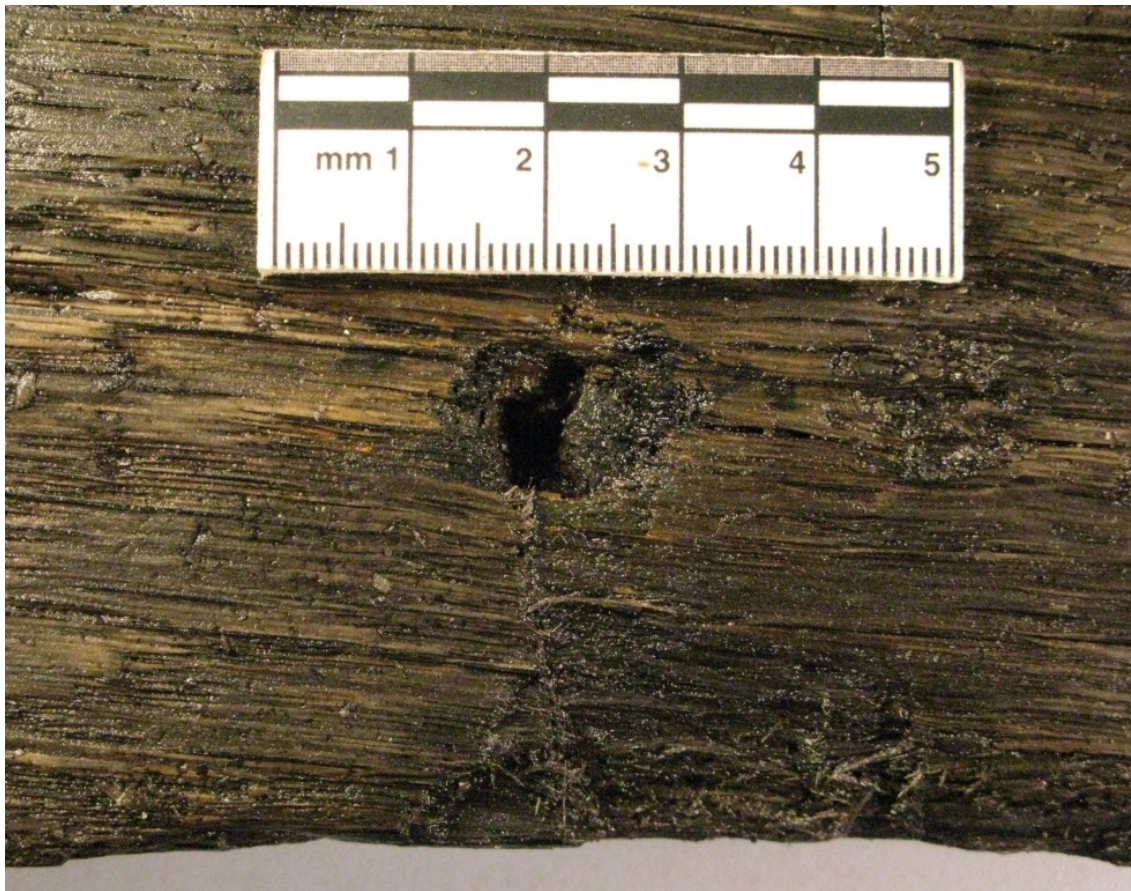
Figure 70 Photograph showing second iron fitting on timber 74
