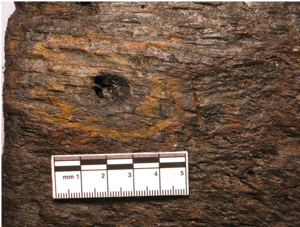
Figure 35 Photograph of Iron fitting and head compression on timber 22
