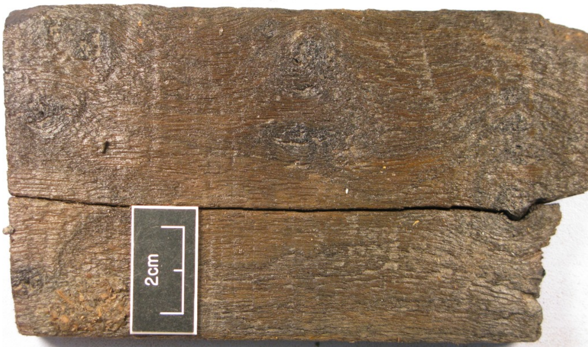
Figure 55 Photograph of saw marks on timber 67
